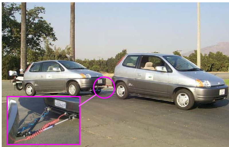
Figure 3. Manual towing to relocate vehicles in the UCR IntelliShare system.
